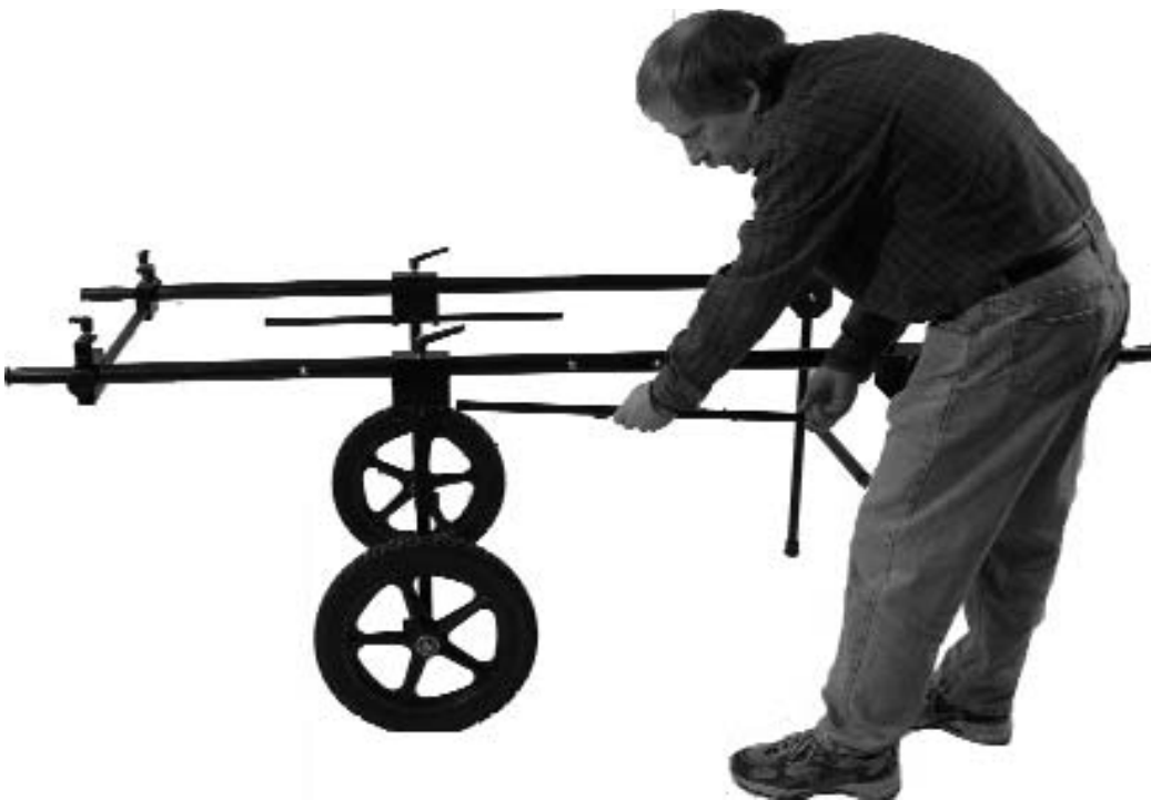
21. Once the Kickstand and Cross Members are installed the Stanchion Support Tubes, used to position the stanchion, can be move from their bottom position to a top position. In the higher position they are out of the way and can be used to hang equipment if desired.
